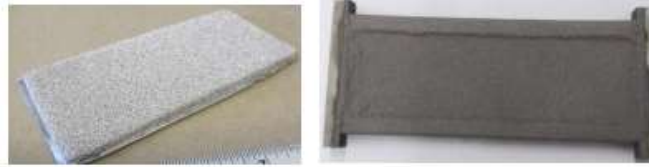
Figure 3: Real images of (a) Metal foam (b) Metal foam heat exchanger after thermal spray coating
